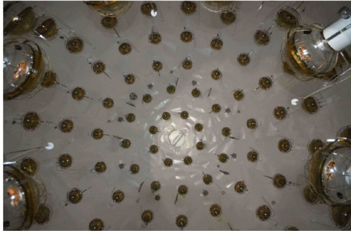
Figure 2.5: Internal view of the LSV neutron veto from its top port with the PMTs directly mounted on the surface of the sphere. Credit: [23]
